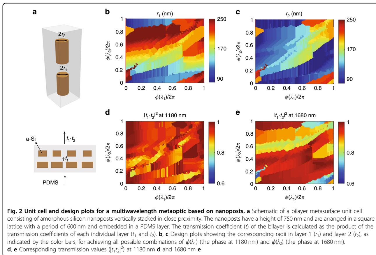
presented in Fig. S2. These design plots can be used to quickly select the structural parameters of each layer to achieve arbitrary and independent phase profiles at the two wavelengths of interest.
