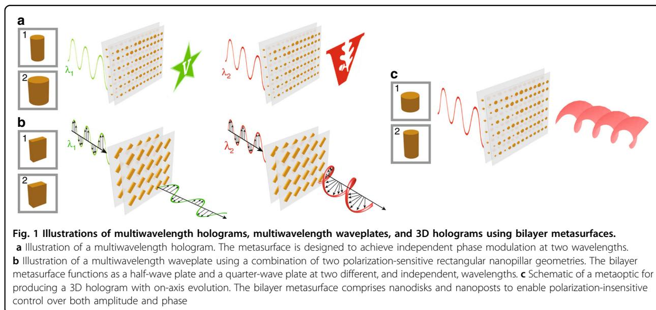
controlled at two different wavelengths. This freedom is used to realize metaoptics with a wide range of functionalities, including multiwavelength holograms, multiwavelength waveplates, and 3D holograms.
